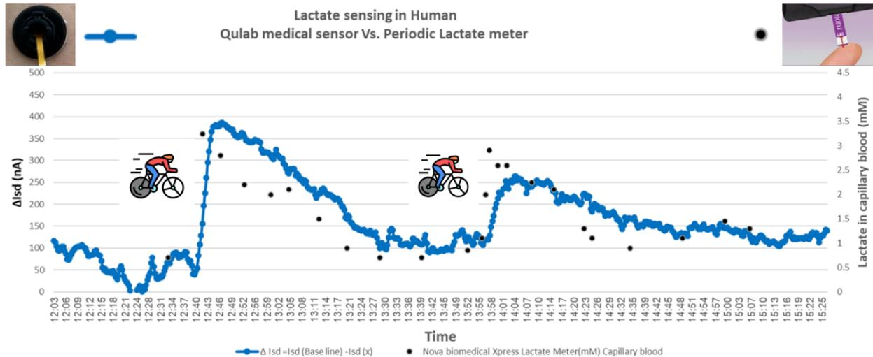
Figure 4. Lactate sensing in human: Representative graph summarizing Lactate sensing results from one Lactate sensor placed on human arm during a period of two rounds of Lactate Threshold Cycling Protocol (blue line) as recorded in  $\Delta$ Isd (nA). Capillary blood Lactate levels as measured periodically using Nova Biomedical Xpress Lactate Meter and presented in mM concentration (black dots).
