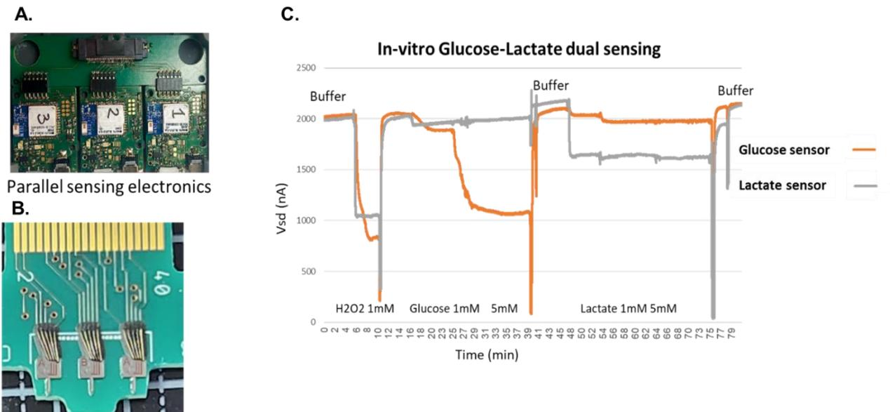
Figure 2. CMM triple parallel electronics for multisensing. A. Three blocks of separate electronic circuits each wired to a single microprobe. B. Enlarged *in-vitro* model of microprobes each connected and wirebonded to an electronic transmitter which allows parallel sensing of different probes. C. Representative graph of dual Glucose-Lactate sensing in parallel, *in-vitro*.
