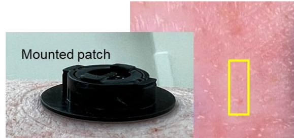
b: Patch #4, microprobes penetration marks on pig skin upon patch removal
